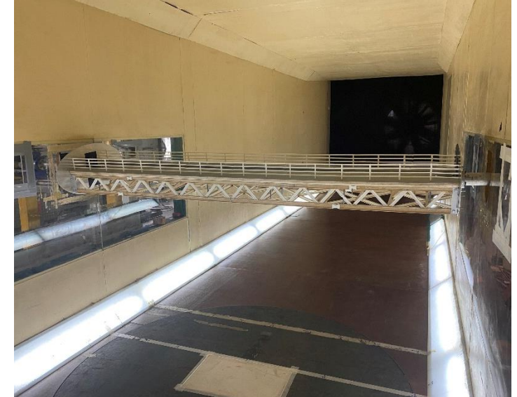
Wind Tunnel Test for Bridges
